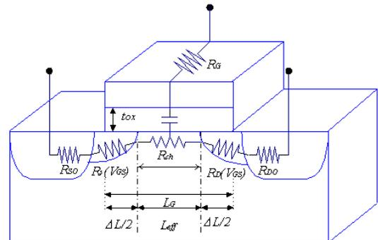
Fig. 1. Cross section and parasitic elements in a MOSFET.
