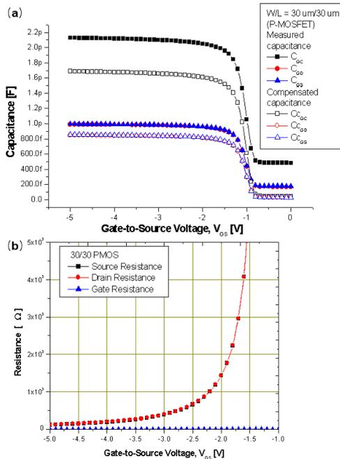
Fig. 6. (a) Compensated capacitances and (b) parasitic resistances in a P-MOSFET with  $W/L = 30 \mu\text{m}/30 \mu\text{m}$ .
