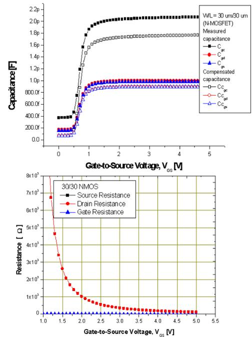
Fig. 5. (a) Compensated capacitances and (b) parasitic resistances in an N-MOSFET with  $W/L = 30 \mu\text{m}/30 \mu\text{m}$ .
