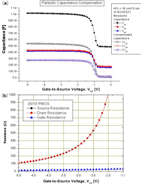
Fig. 8. (a) Compensated capacitances and (b) parasitic resistances in a P-MOSFET with  $W/L=30 \mu\text{m}/10 \mu\text{m}$ .
