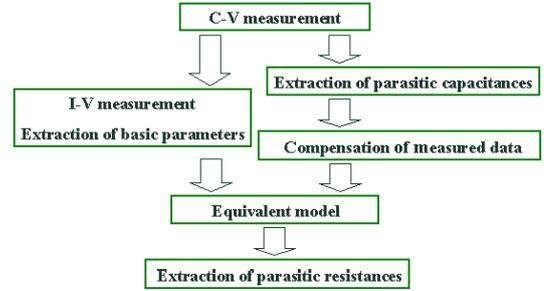
Fig. 4. Flow chart for extracting device parameters in MOSFETs combining the C-V and I-V measurements.
