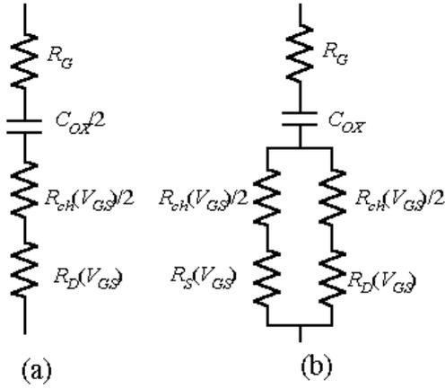
Fig. 3. Equivalent circuits for the (a) gate-to-drain admittance and the (b) gate-to-channel (source-drain-connected) admittance.
