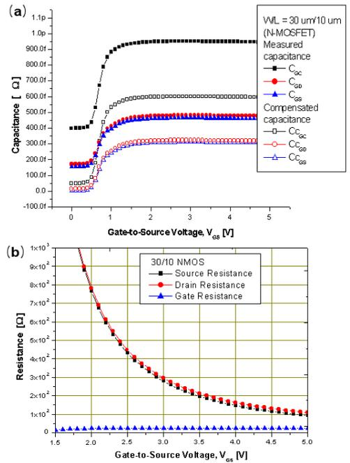
Fig. 7. (a) Compensated capacitances and (b) parasitic resistances in an N-MOSFET with  $W/L = 30 \mu\text{m}/10 \mu\text{m}$ .
