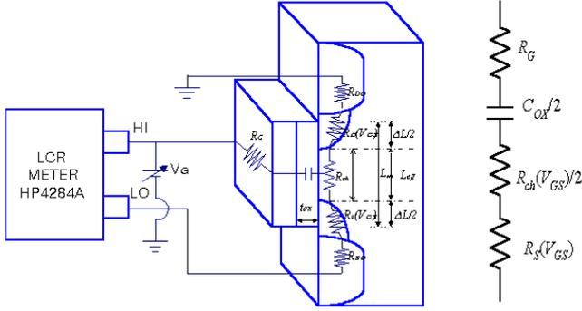
Fig. 2. Schematic diagram and equivalent circuit for the C-V measurement.
