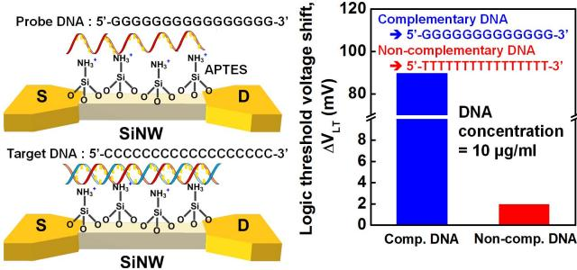
**Fig. 16:** Experimental procedures for DNA detection using the electrostatic immobilization method.
