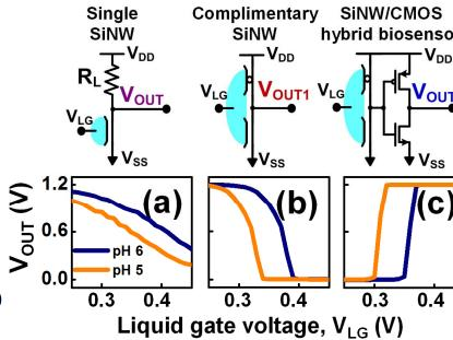
**Fig. 12:** Voltage transfer curves of (a) the resistive load type (single SiNW), (b) complementary SiNW block (1<sup>st</sup> stage), and (c) SiNW/CMOS hybrid biosensor (1<sup>st</sup> and 2<sup>nd</sup> stages). (d) A comparison of output voltage sensitivities in three types of biosensors ( $V_{DD} = 1.2$  V).
