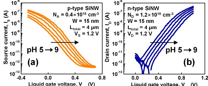
**Fig. 7:** Transfer characteristics of (a) p-type and (b) n-type SiNW FETs for different pH levels (0.1 M potassium phosphate buffer, pH 5 - 9). An Ag/AgCl reference electrode was employed as the liquid gate voltage ( $V_{LG}$ ) electrode. As the pH changed, a clear threshold voltage shift and current modulation was observed for both n- and p-type FETs.
