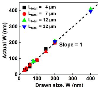
**Fig. 6:** SiNW W versus the actual SiNW W of fabricated SiNWs on a SOI wafer. The actual SiNW W was extracted from the SEM images.
