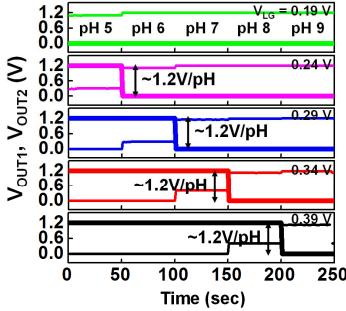
**Fig. 11:** Transient responses of the output voltages due to changes in the pH level in the SiNW/CMOS hybrid biosensor (thick line:  $V_{OUT2}$ , thin line:  $V_{OUT1}$ ).
