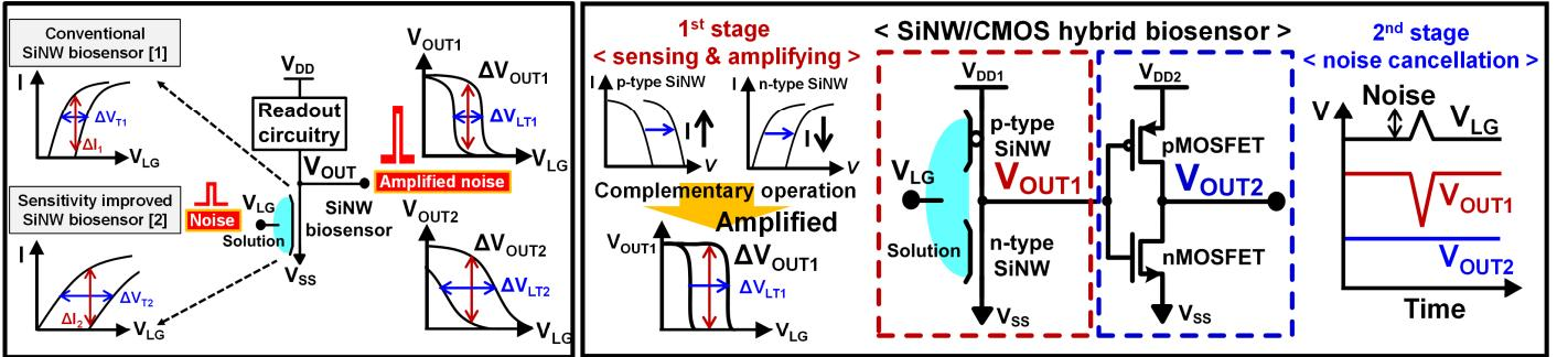
**Fig. 1:** Previous studies [1, 2] on biosensors showed an increase in the  $V_T$  shift, but the current sensitivity did not change ( $\Delta V_{T1} < \Delta V_{T2}$ ,  $\Delta I_1 = \Delta I_2$  [3]). Accordingly, the output voltage sensing margin in the actual readout circuitry did not improve ( $\Delta V_{OUT1} = \Delta V_{OUT2}$ ). Moreover, noise or fluctuations could be amplified.
