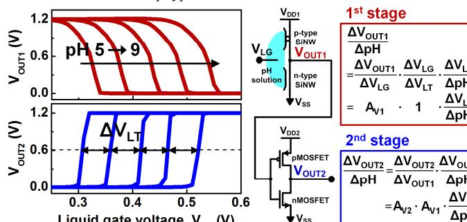
**Fig. 10:** (Left) Output voltage sensitivity of the 1<sup>st</sup> and 2<sup>nd</sup> stages of the SiNW/CMOS hybrid biosensor. (Right) Measured voltage transfer curves and extracted voltage gains of the SiNW/CMOS hybrid biosensor.
