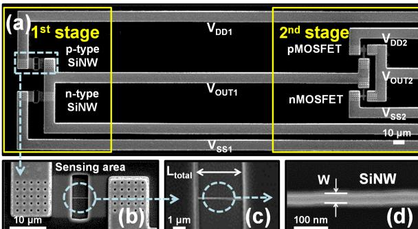
**Fig. 4:** Scanning electron microscopy images of (a) the SiNW/CMOS hybrid biosensor. (b) A SiNW biosensor in the 1<sup>st</sup> stage. (c) Magnified view ( $L_{total} = 4$   $\mu$ m). (d) SiNW channel region.
