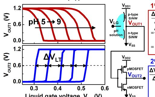
**Fig. 8:** Threshold voltage shift ( $\Delta V_T$ ) with respect to pH changes for both n- and p-type SiNW FETs. The average  $\Delta V_T$  per pH remained below the Nernst limit (59.6 mV/pH @  $T = 300$  K).
