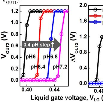
**Fig. 14:** Measured voltage transfer curves of the SiNW/CMOS hybrid biosensor for different pH values in increments of 0.4 units. The averaged  $\Delta V_{OUT2}/0.4$  pH was approximately 1.2 V.
