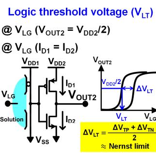
**Fig. 9:** (Left) Definition of the logic threshold voltage ( $V_{LT}$ ) and its influence on the threshold voltage shift due to pH changes. (Right) Measured voltage transfer curves of the SiNW/CMOS hybrid biosensor for different pH levels ( $W = 15$  nm,  $L_{total} = 4$   $\mu$ m,  $V_{DD1} = V_{DD2} = 1.2$  V). The average  $\Delta V_{LT}$  was 53.5 mV.
