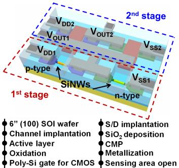
**Fig. 3:** Process flow of the SiNW/CMOS hybrid biosensor on a SOI wafer.
