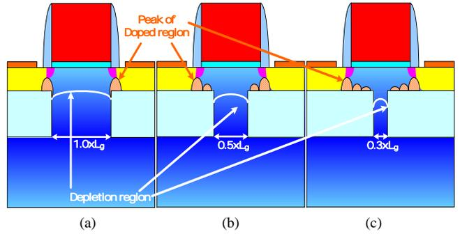
Fig. 3. The relation between the location of the halo doped region and the  $L_{PiOX}$ . (a)  $L_{PiOX}=1.0 \times L_g$ . (b)  $L_{PiOX}=0.5 \times L_g$ . (c)  $L_{PiOX}=0.3 \times L_g$ .
