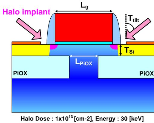
Fig. 1. The schematic diagram of simulated PiFET.
