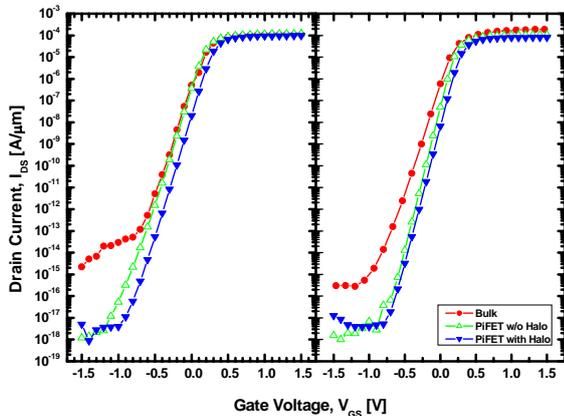
Fig. 2. The  $I$ - $V$  characteristics of PiFET, bulk MOSFETs, and SOI MOSFET with  $L_g=30$  and  $50$  nm, respectively.
