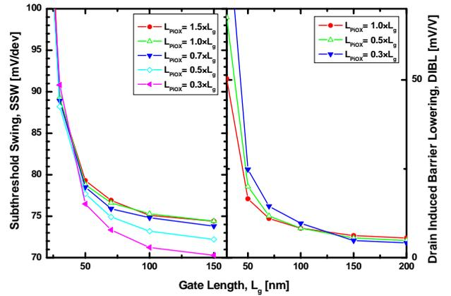
Fig. 4. The  $L_{PiOX}$ -dependence of both SSW and DIBL.
