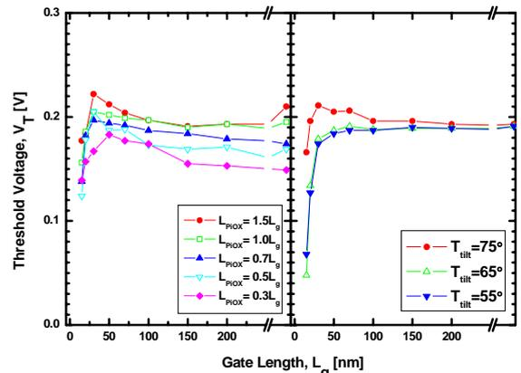
Fig. 6. The  $V_T$  roll-off characteristic of PiFET. (a) The  $L_{PiOX}$ -dependence at a fixed  $T_{tilt}=75^\circ$ . (b) The  $T_{tilt}$ -dependence of the reverse SCE.
