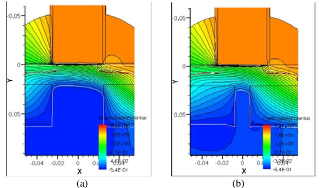
Fig. 5. Potential contour distribution at the  $V_D=1.5$  V. (a)  $L_{PiOX}=1.0 \times L_g$ . (b)  $L_{PiOX}=0.3 \times L_g$ . As the  $L_{PiOX}$  increases, the DIBL decreases.
