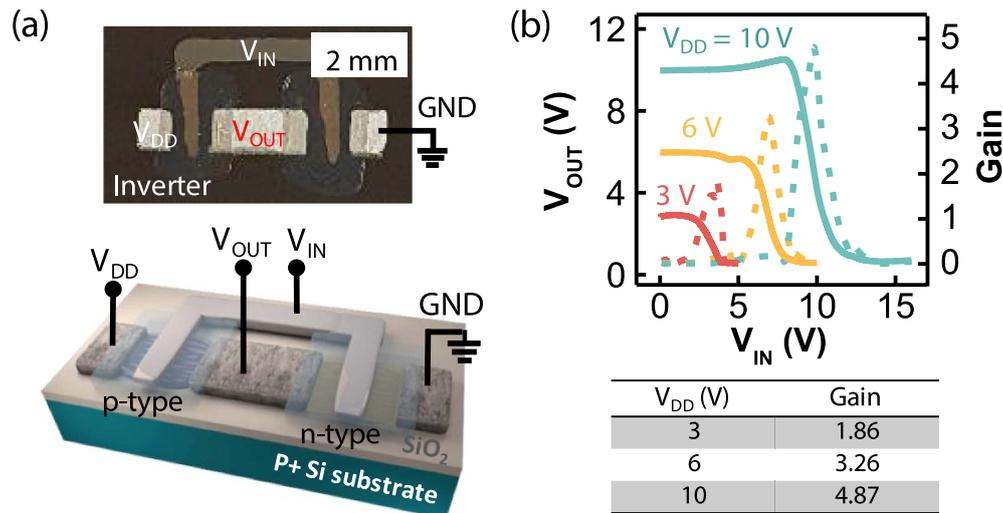
**Figure 4.** (a) Optical image of the drawn complementary inverter consisting of the drawn p-type CNT-TFT and the drawn n-type CNT-TFT with a  $L$  of 2 mm, a  $W$  of 2 mm, and a  $L_G$  of 1 mm. (b) Voltage transfer characteristics of the drawn complementary inverter (solid lines) and voltage gain ( $IdV_{OUT}/dV_{IN}$ ) obtained from the voltage transfer curves (dashed lines), where  $V_{DD}$  values of 3 V, 6 V, and 10 V were applied.
