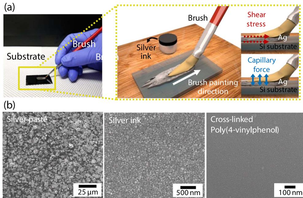
**Figure 1.** (a) Image showing silver ink directly drawn on a Si substrate with a brush and schematics showing the process and principle of the direct drawing method for fabricating a film of the silver ink. (b) Surface SEM images of the drawn films of solution-based materials, including silver paste, silver ink, and cPVP.
