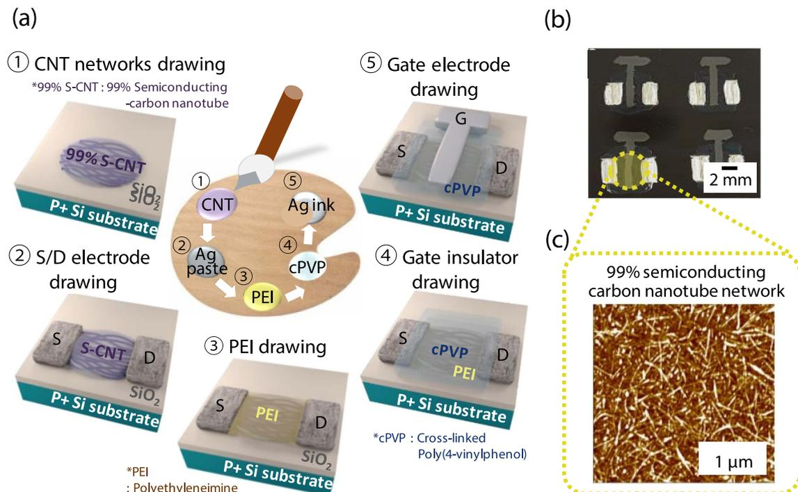
**Figure 2.** (a) Process flow of the drawn top-gate CNT-TFT in which the CNT network was doped with the strongly electron-donating PEI polymer. (b) Optical image showing an array of drawn CNT-TFTs with a L of 2 mm, a W of 2 mm, and a L<sub>G</sub> of 1 mm. (c) AFM image of the solution-processed 99% semiconducting CNT network deposited by the direct drawing method using a brush.
