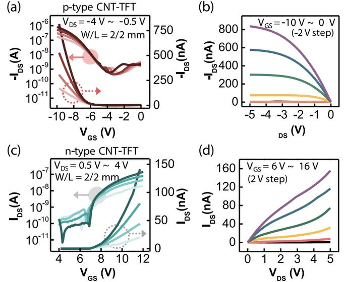
**Figure 3.** (a) Transfer characteristics ( $I_{DS}$ – $V_{GS}$ ) at various  $V_{DS}$  values and (b) output characteristic ( $I_{DS}$ – $V_{DS}$ ) at various  $V_{GS}$  values of the drawn p-type CNT-TFT without the PEI doping treatment. (c) Transfer characteristics at various  $V_{DS}$  values and (d) output characteristics at various  $V_{GS}$  values of the drawn n-type CNT-TFT with the PEI doping treatment.
